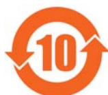
Figure 4 China RoHS label (original colour is orange-red): EFUP label (content of SJ/T11364—2006)
